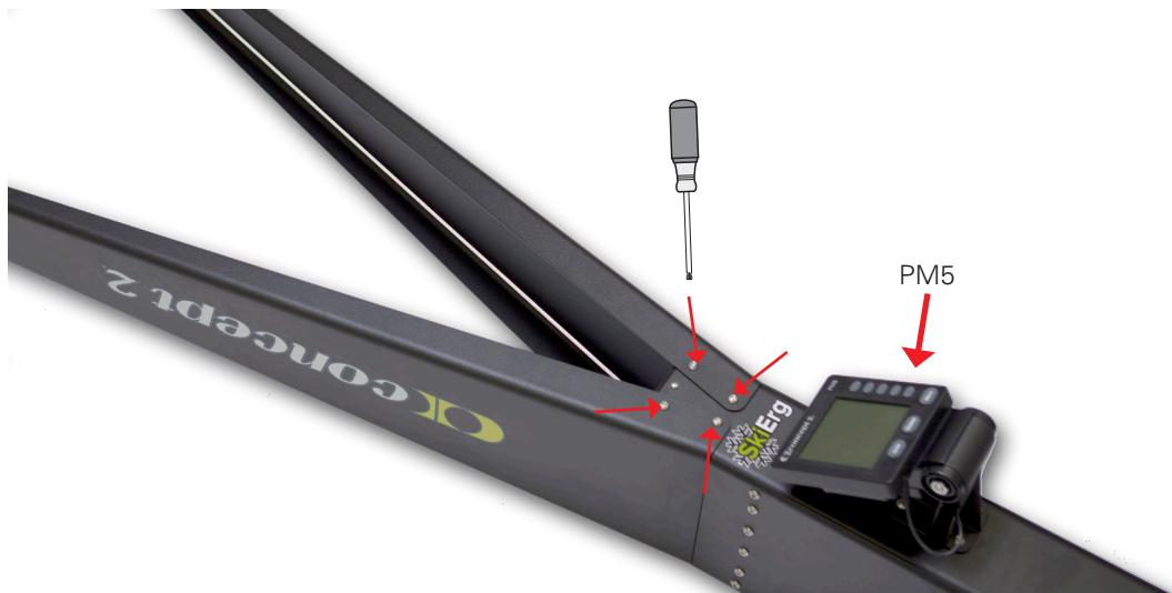
**EN** With the flywheel and PM5 facing up as shown, attach the upper arms to the front side of the SkiErg body using four fasteners.
