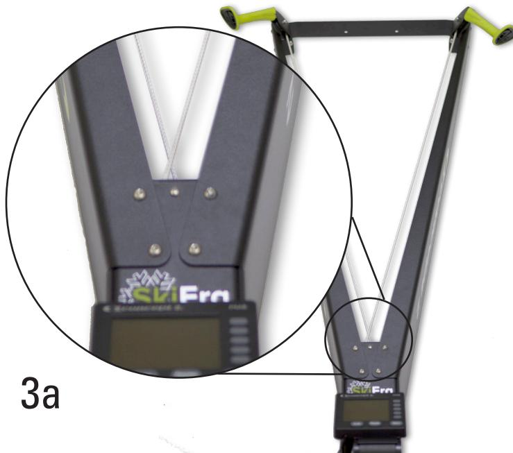
**EN** Attach the top bracket to the tops of the arms using four fasteners—2 fasteners per side. The white handle cords should be crossed once as shown in photo 3a. Remove the shipping insert on the white handle cords to release.
